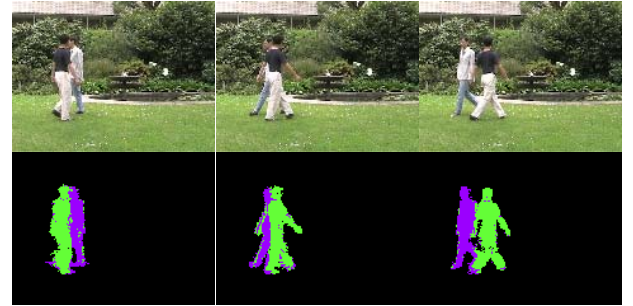
Figure 2. Segmentation results according to Equation (4). The first row: original images (frame numbers from the left column to the right column are 227, 228 and 229); The second row: human segmentation results;
