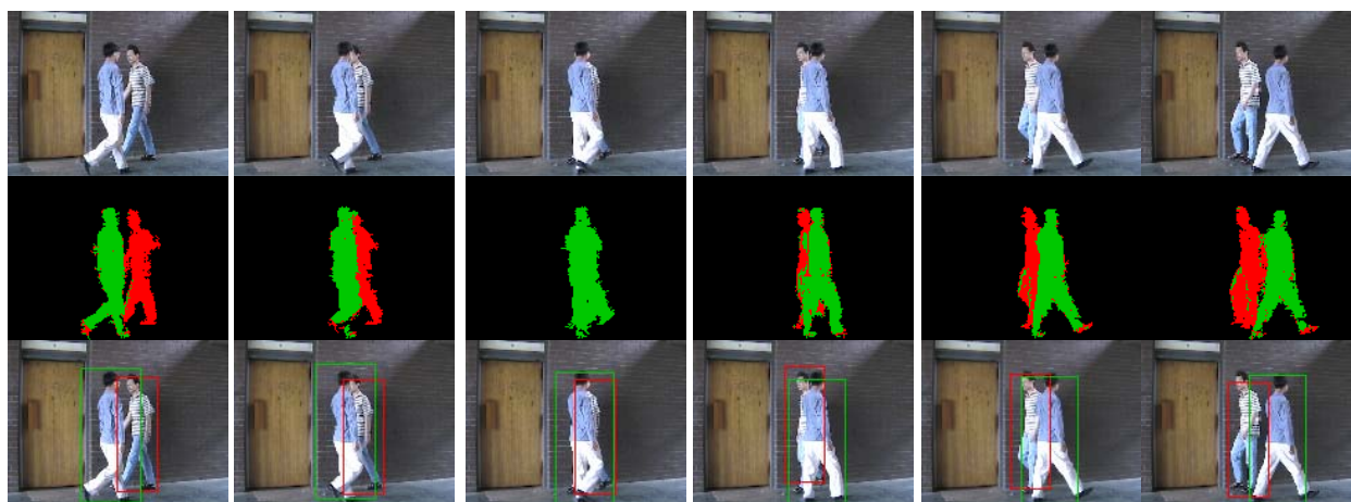
Figure 3. Segmentation and tracking results. The first row: original images (frame numbers from the left column to the right column are 103 to 108); The second row: human segmentation results; The third row: tracking results.
